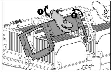
Figure 1-16: Removing the processor cage
